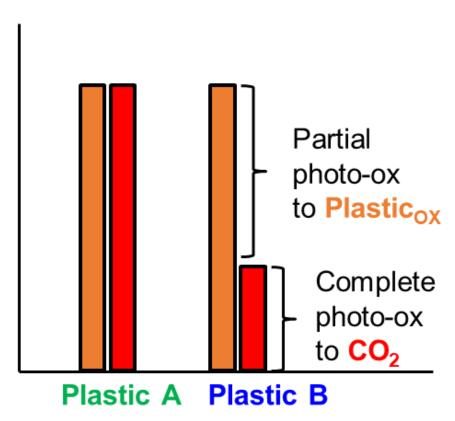
Plastic B is more susceptible to partial photo-oxidation than Plastic A
